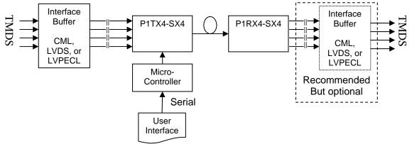
The input to the P1TX4A-SX4-01 must be AC-coupled. The output from the P1RX4A-SX4-01 is CML.
